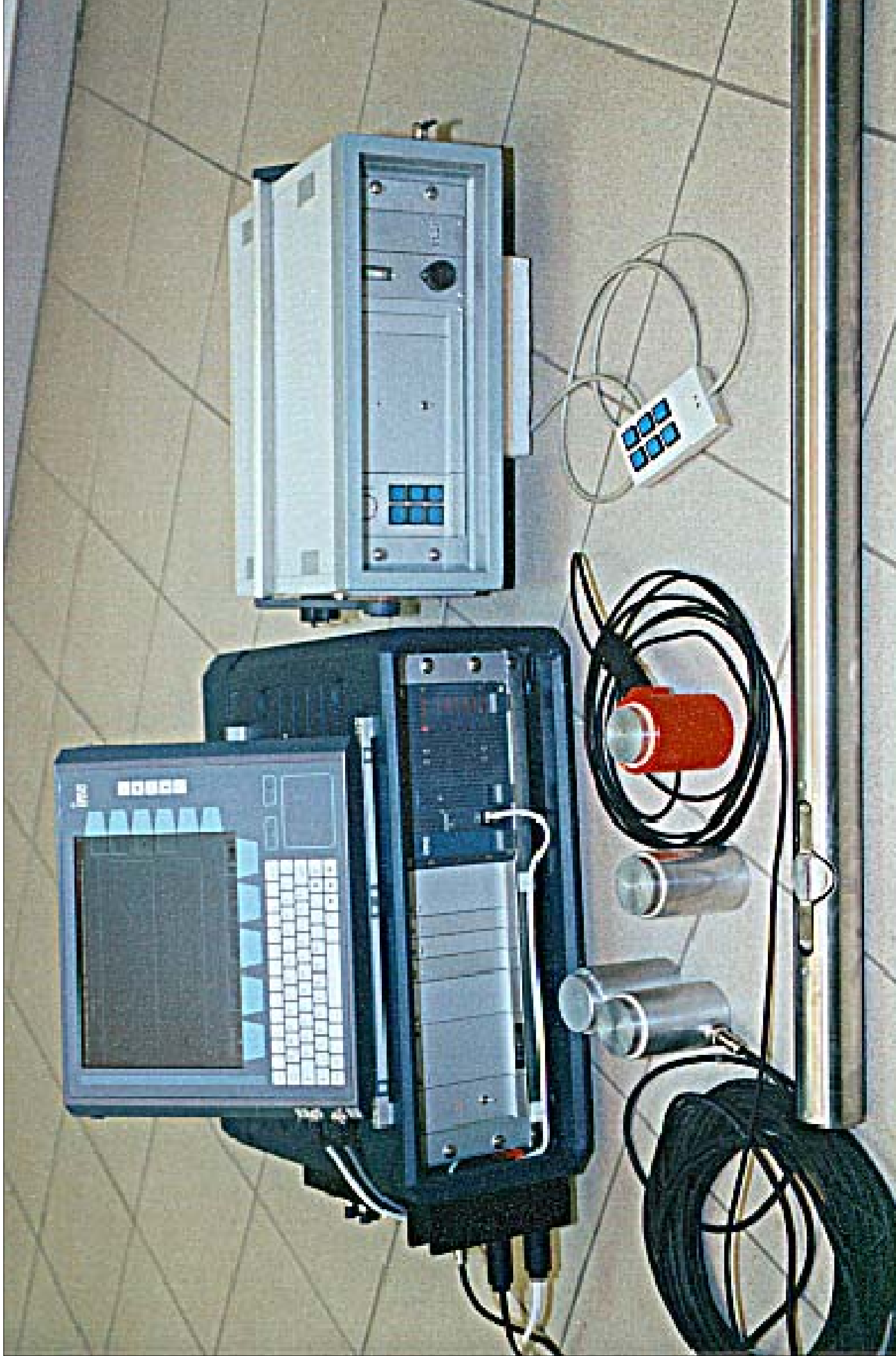
The ultrasonic-seismic measuring system KUTEC 4 with transmitter, receiver and borehole probe
