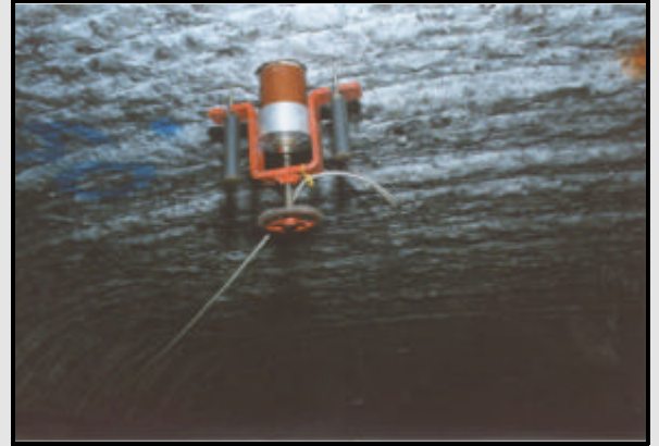
Transmitter coupled to the salt rock
