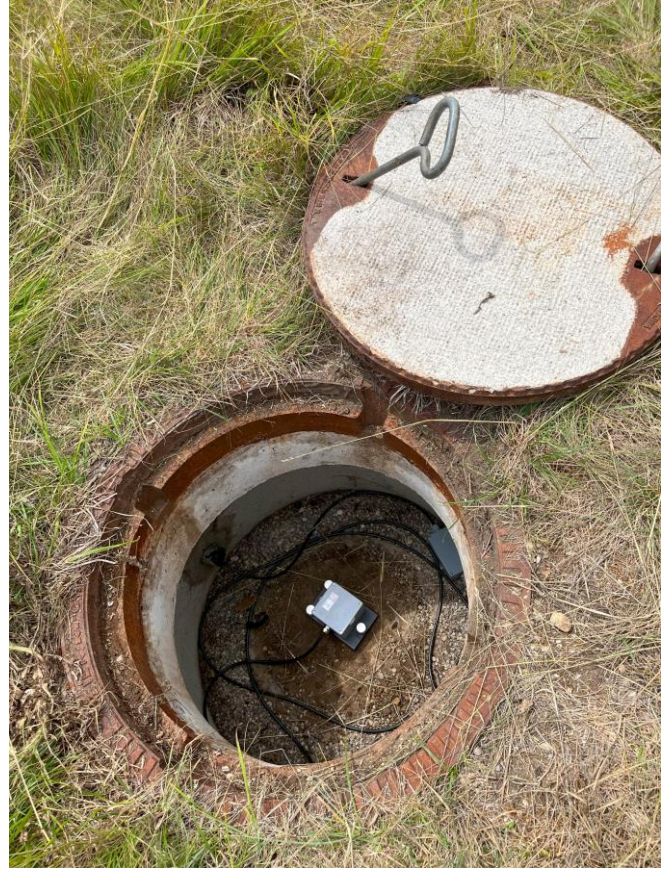
Seismometer at surface
