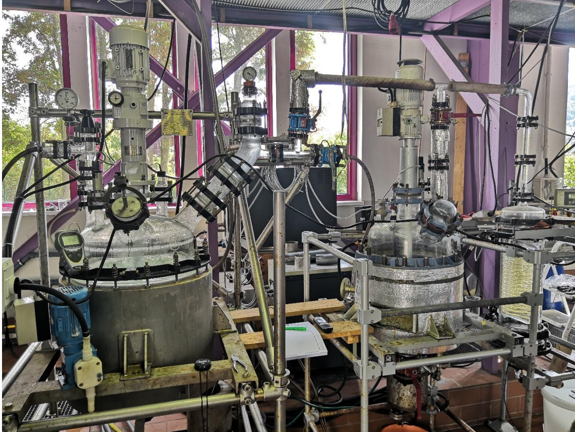
Evaporation crystalliser (left) and salt crystallising unit (right)
