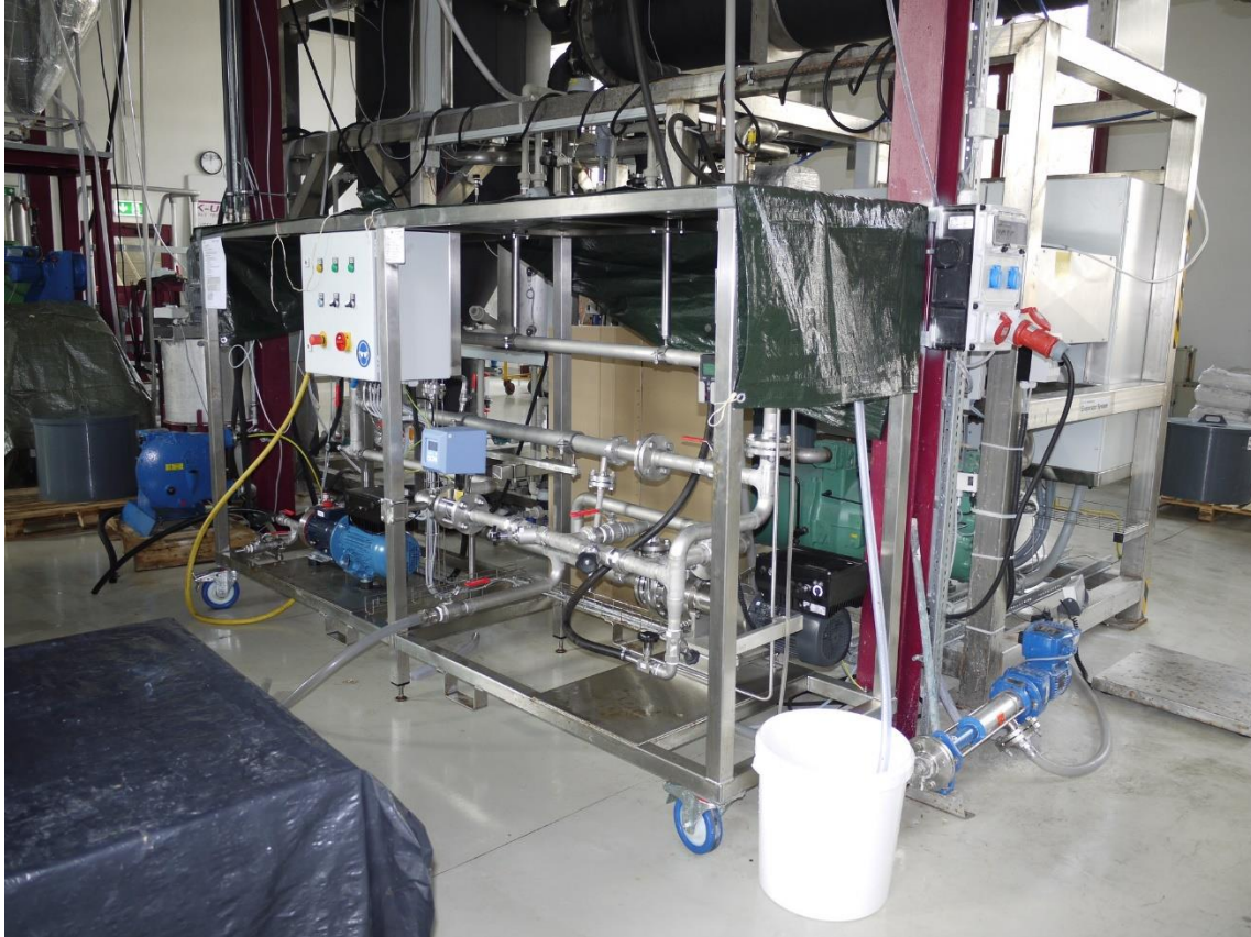
NF and RO plant (left) and IEx column (right)
