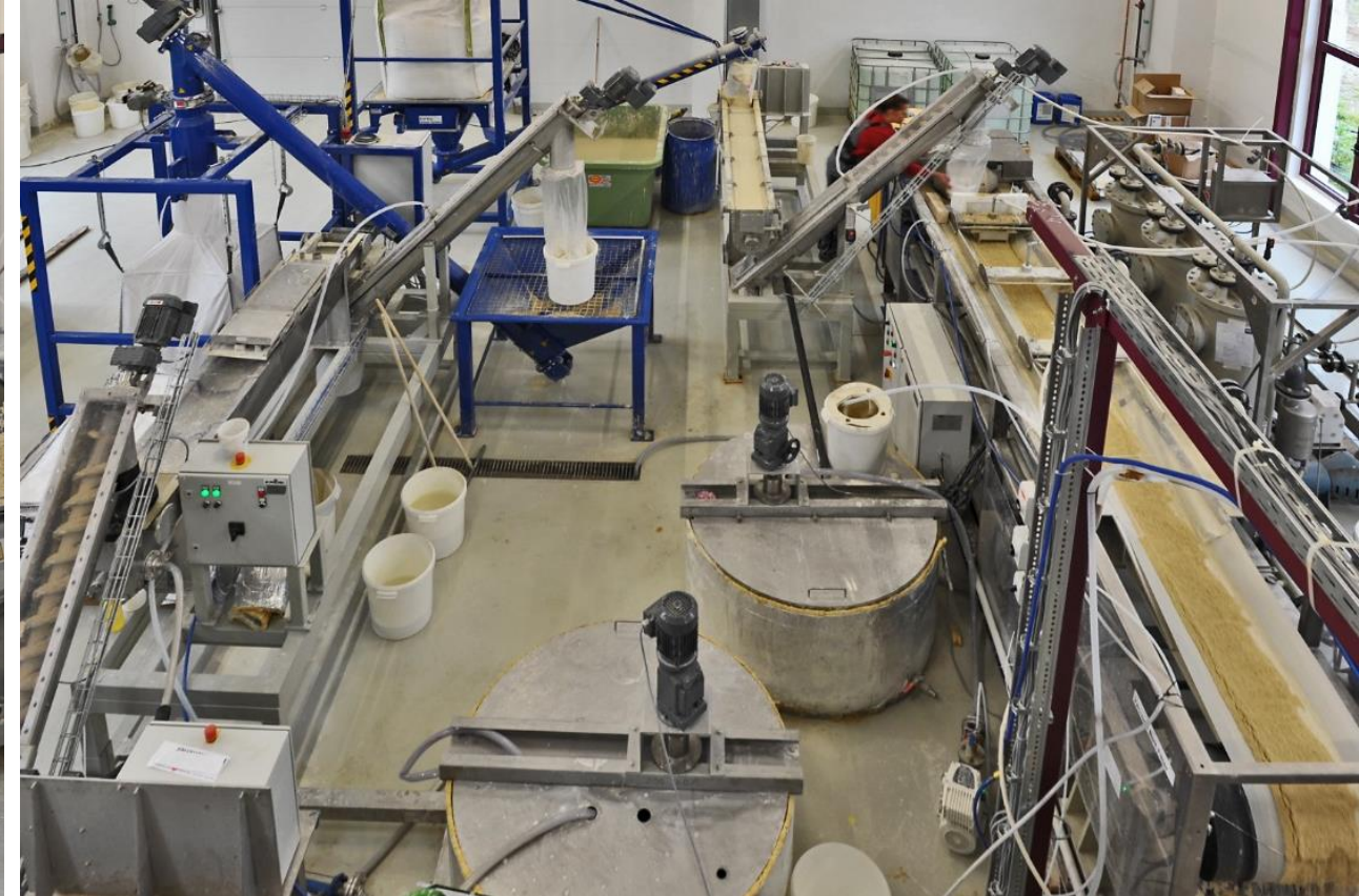
Top view dissolver and belt filter
